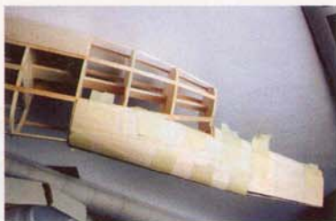
Sheeting the rear portion
