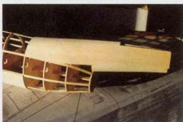
Completed sheeting on rear portion
